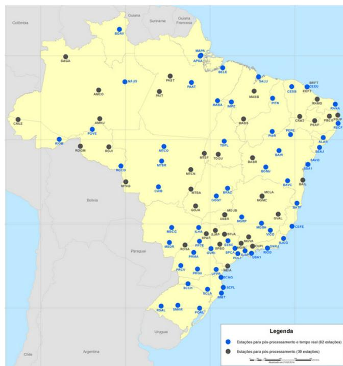
**Figure 4. Stations configuration of RBMC. Blue points: real time stations; black points: post-processed stations. Image from IBGE website, available at <[http://www.ibge.gov.br/home/geociencias/geodesia/rbmc/rbmc\\_est.php](http://www.ibge.gov.br/home/geociencias/geodesia/rbmc/rbmc_est.php)>.**
