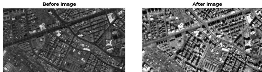
Figure 3. Images of the differences in brightness and contrast between bands 1 (left) and 4 (right) of the CBERS-4A satellite image from 2021.
